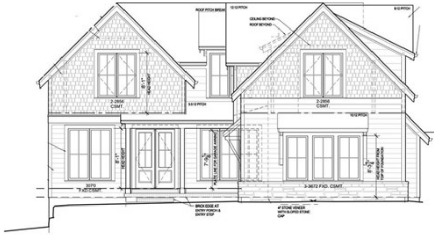
FRONT ELEVATION SCALE 1/4" = 1'-0"
